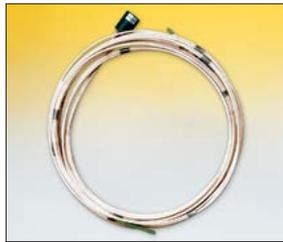
**Model 1280 (A-6) Flexible Rod Extensometer**
