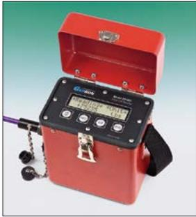
**Model GK-502 Load Cell Readout**
